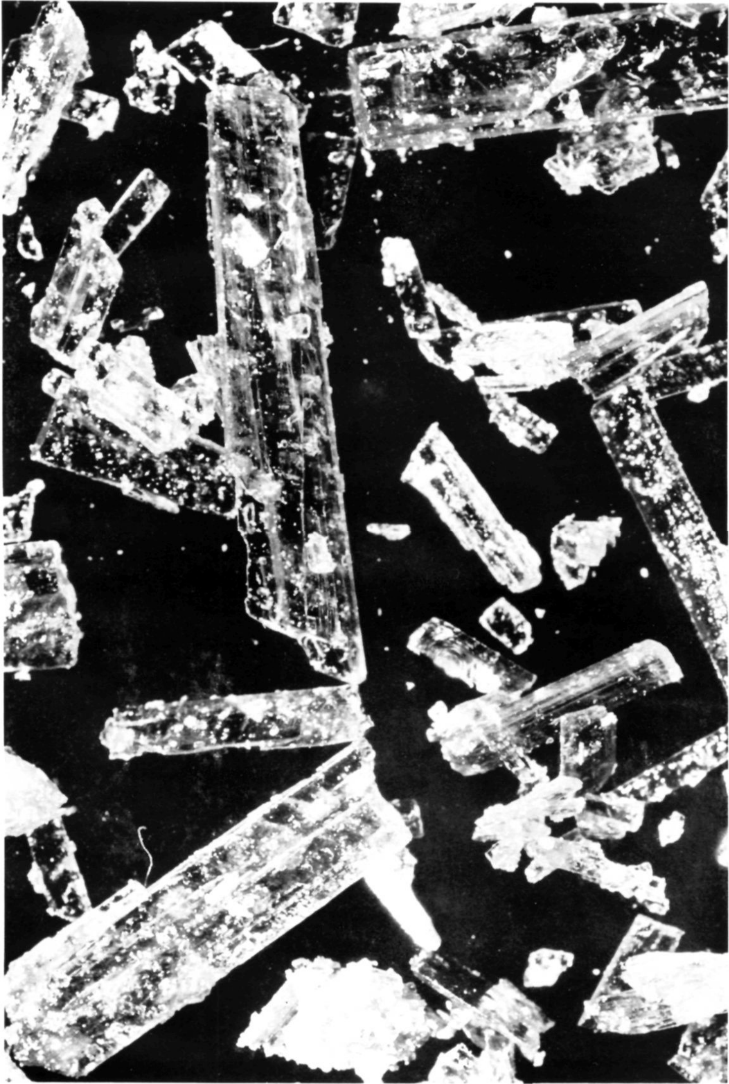
Fig. 1.—Crystalline vitamin A, m. p. 63–64°, \times 14 . (Photomicrographs, Figs. 1 and 2, courtesy of R. P. Loveland, Eastman Kodak Company, Research Laboratories.)
